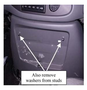
**3.** Remove mount brackets from console housing and attach to engine cover with  $\frac{1}{4}$ " x 1  $\frac{1}{4}$ " hex head bolts, stop nuts and fender washers.
